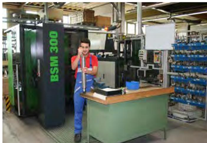
The Dr. Fritsch BSM 300 for laser welding core bits from from 3.5 inches to 12 inches (8 mm to 305 mm).
