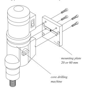
Then fasten the assembled unit onto carriage with four socket had cap screws.
