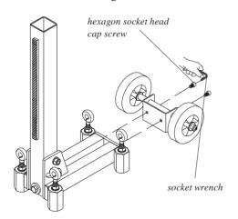
Push the gearbox onto the shaft and fastening it with the hexagon socket head cap screw. You can fasten the gearbox from both sides, also the cross handle.
